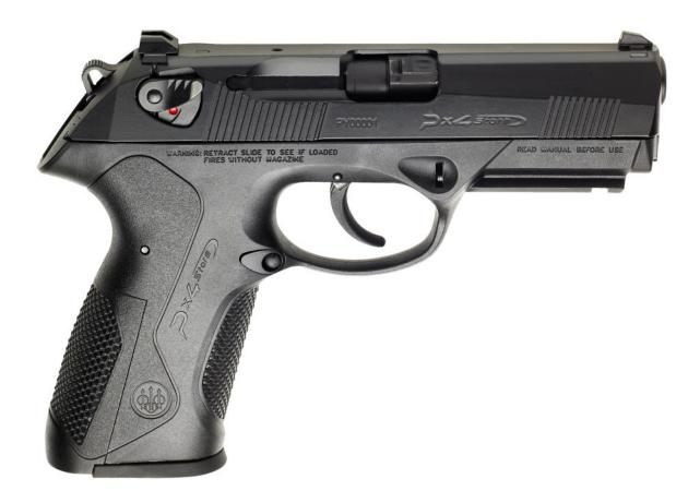
Manufactured in three calibers, the PX4 Storm features a locked-breech with a rotating barrel system, the strongest action to date. The light yet durable frame employs modern thermoplastic technology through the use of polymer reinforced fiberglass. The modular structure, versatility, and ergonomics of the PX4 Full size make it the ideal firearm for the professional user.
