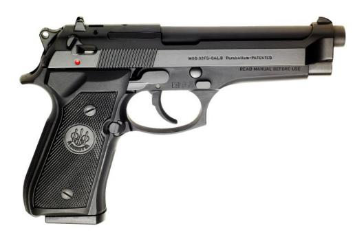
The Beretta 92FS is a double/single-action semiautomatic pistol that employs an open-slide, short-recoil delayed locking-block system, which yields a faster cycle time and delivers exceptional accuracy and reliability. In particular, the open-slide design practically eliminates "stove-piping" and helps flawless cycling and feeding even after thousands of rounds. The 92FS reversible magazine release and ambidextrous safety-decocker make it flexible for right- or left-handed operators.
