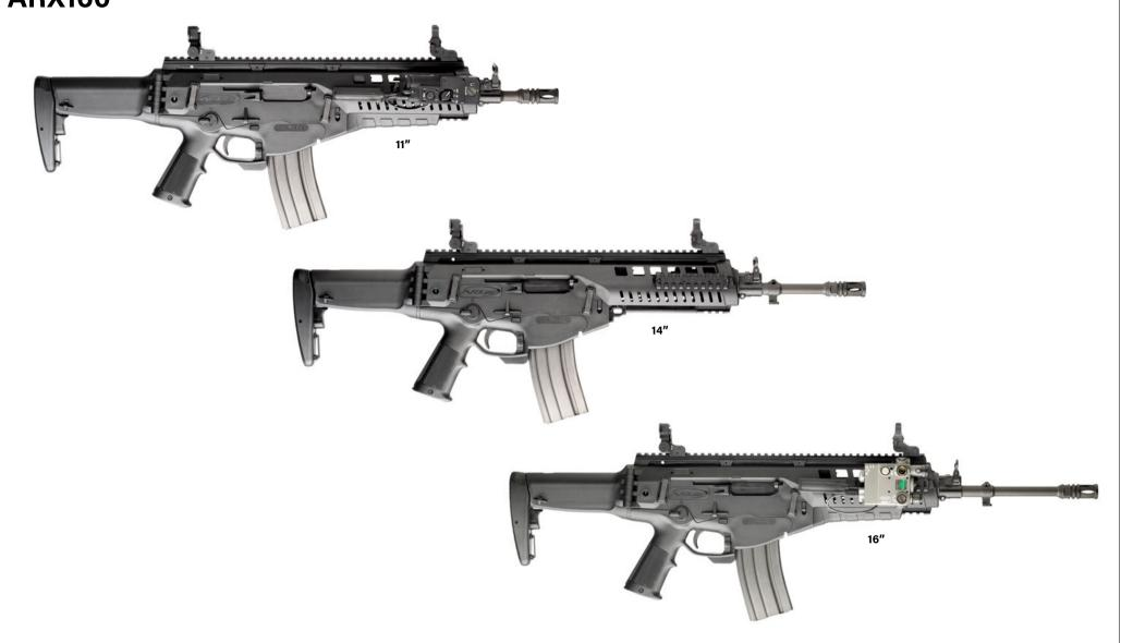
**Product:** The automatic rifle ARX 160 consists of a rifle and a 30 rounds magazine cal. 5.56 x 45 mm NATO. The rifle may be configured with barrel lengths of 11, 14 and 16 inches, respectively; ARX 160 features a quick-change barrel, so that to be removed and installed in a few seconds without tools. It is a gas-operated, locked breech rotating bolt weapon, that can be fired either in burst or single shots.
