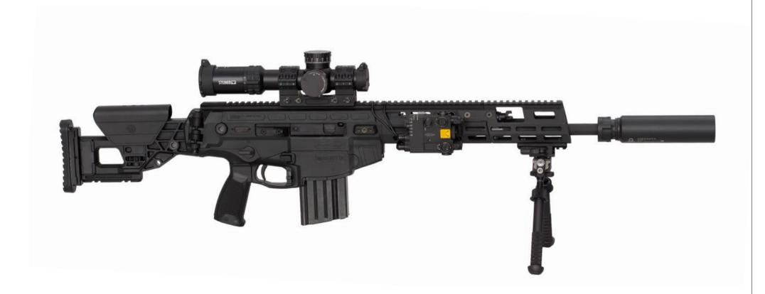
**Product:** The semiautomatic rifle ARX200 DMR, cal 7,62x51 NATO is a gas operated, locked breech rotating bolt weapon. Rifle is offered with 16 or 20 inches barrel lengths. Accuracy with match ammunition is around 1 MOA.
